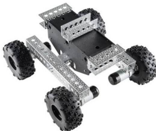
Figure 12: Rectangular chassis with four wheels.
