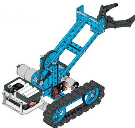
Figure 14: Horizontal pick and place armed gripper placed on the back-end of the robot
